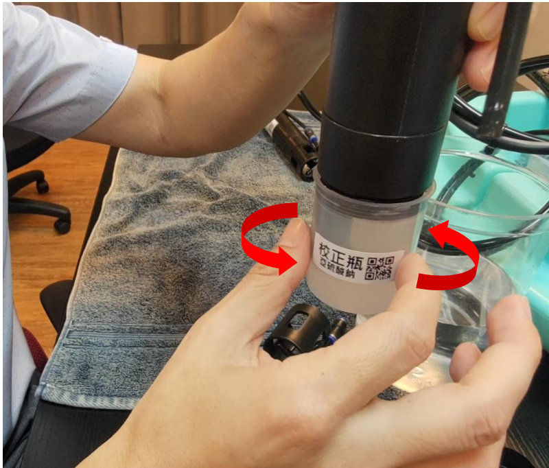
Install NaNO 2 calibration bottle
